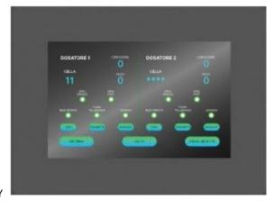
**CALIBRATION FUNCTIONS**, WHICH ALLOW THE USE OF VARIOUS TYPES OF LOAD CELLS WITH DIFFERENT FLOW RATES, IN ORDER TO MEET ALL REQUIREMENTS OF SPEED, ACCURACY AND PRECISION.
